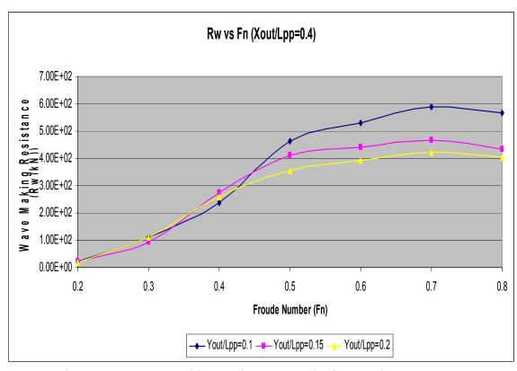
Figure 15. Wave Making Resistance Results for  $X_{out}/L_{pp} = 0.4$
