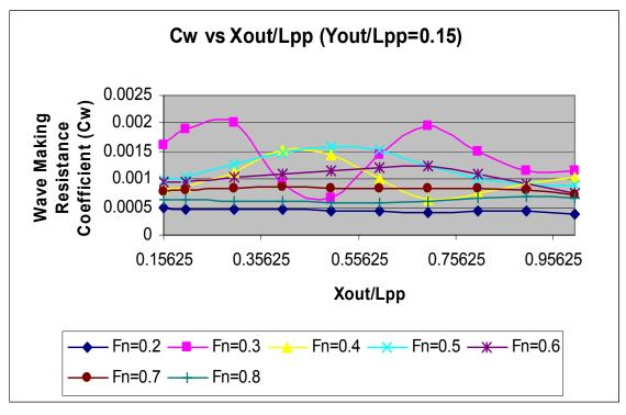
Figure 57. Wave Making Resistance Coefficient Results for  $Y_{out}/L_{pp} = 0.15$
