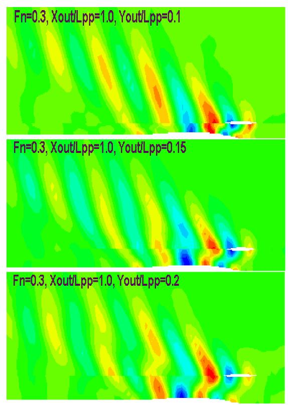
Figure 39. Wave Pattern for  $X_{out}/L_{pp} = 1.0$ , at Froude Number 0.3
