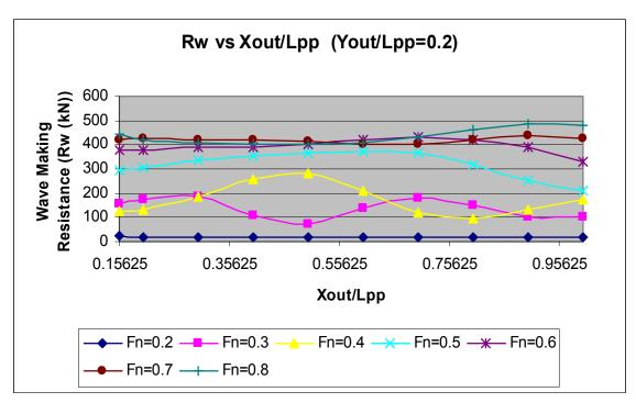
Figure 60. Wave Making Resistance Results for  $Y_{out}/L_{pp} = 0.2$
