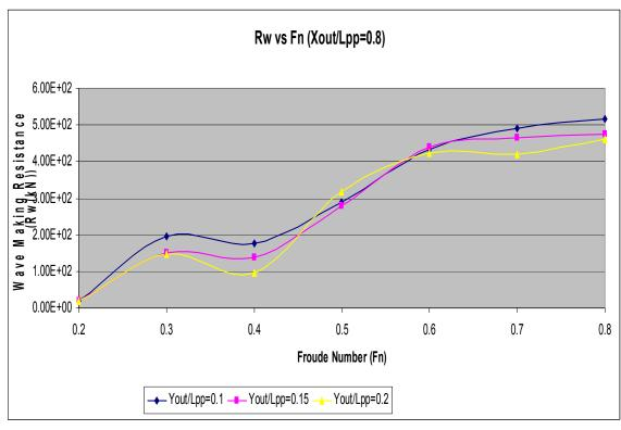
Figure 23. Wave Making Resistance Results for  $X_{out}/L_{pp} = 0.8$
