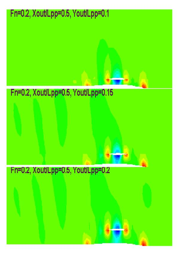
Figure 35. Wave Pattern for  $X_{\it out}$  /  $L_{\it pp}$  = 0.5 , at Froude Number 0.2
