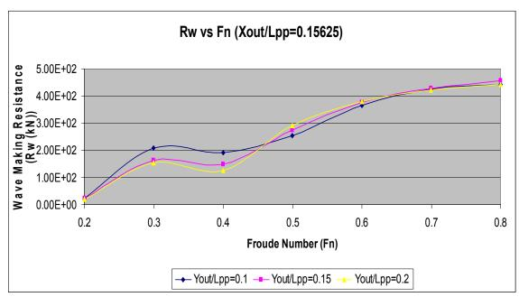
Figure 9. Wave Making Resistance Results for  $X_{out}/L_{pp} = 0.15625$
