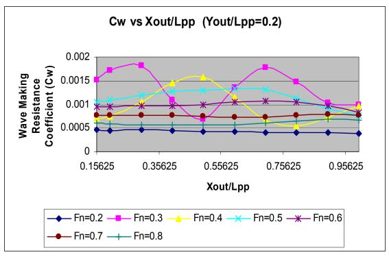
Figure 59. Wave Making Resistance Coefficient Results for  $Y_{out}$  /  $L_{pp}$  = 0.2
