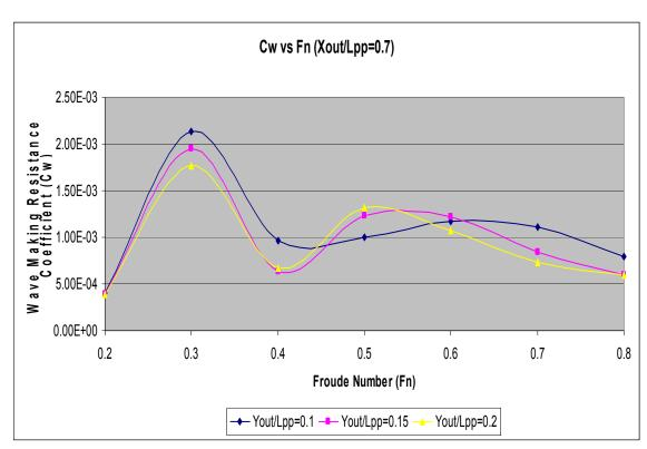
Figure 20. Wave Making Resistance Coefficient Results for  $X_{out}/L_{pp} = 0.7$
