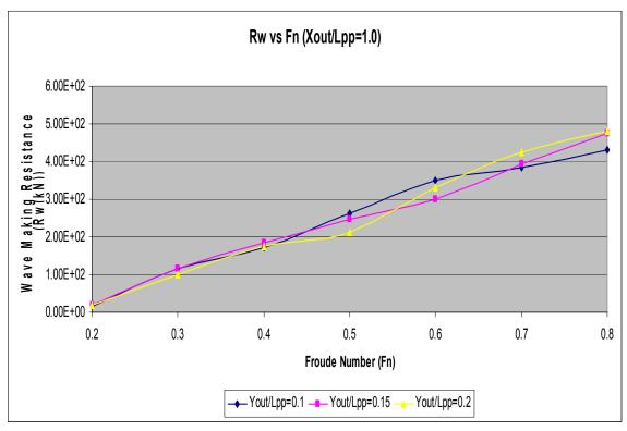
Figure 27. Wave Making Resistance Results for  $X_{out}/L_{pp} = 1.0$
