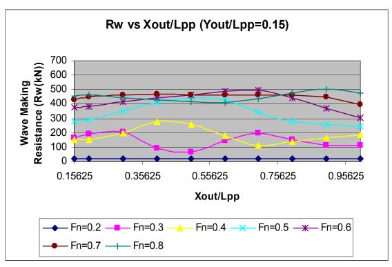
Figure 58. Wave Making Resistance Results for  $Y_{out}/L_{pp} = 0.15$
