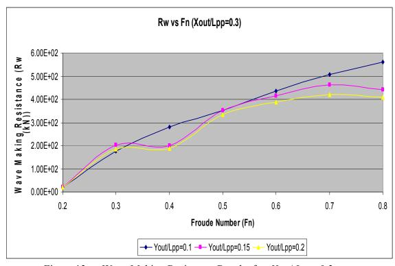
Figure 13. Wave Making Resistance Results for  $X_{out}/L_{pp} = 0.3$
