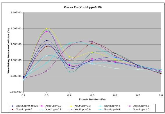
Figure 30. Wave Making Resistance Coefficient Results for  $Y_{out}/L_{pp} = 0.15$
