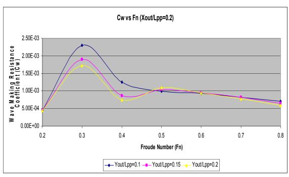
Figure 10. Wave Making Resistance Coefficient Results for  $X_{out}/L_{pp} = 0.2$
