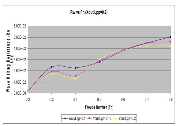
Figure 11. Wave Making Resistance Results for  $X_{out}/L_{pp} = 0.2$
