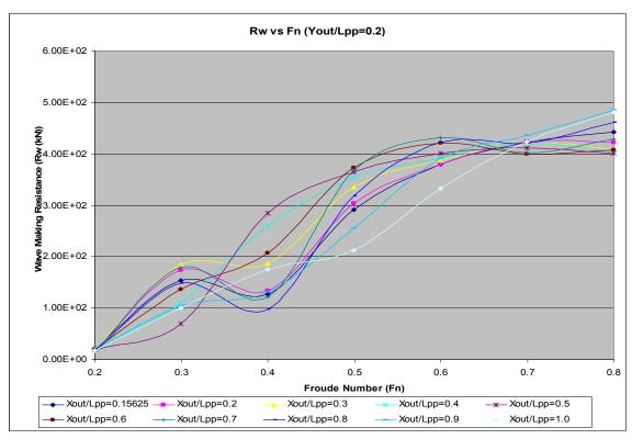
Figure 33. Wave Making Resistance Results for  $Y_{out}/L_{pp} = 0.2$
