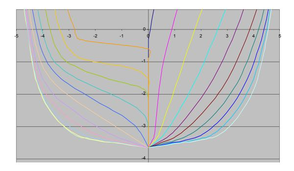
Figure 5. Body Plan of the Main Hull
