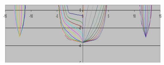
Figure 7. Body Plan of the Trimaran
