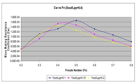
Figure 14. Wave Making Resistance Coefficient Results for  $X_{out}/L_{pp} = 0.4$
