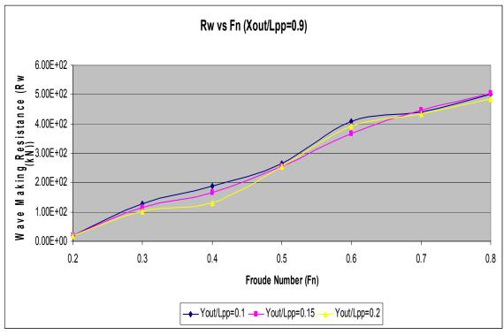
Figure 25. Wave Making Resistance Results for  $X_{out}/L_{pp} = 0.9$
