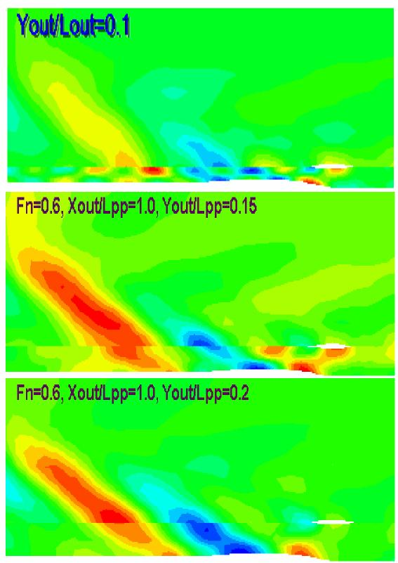
Figure 48. Wave Pattern for  $X_{out}/L_{pp} = 1.0$ , at Froude Number 0.6
