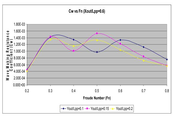
Figure 18. Wave Making Resistance Coefficient Results for  $X_{out}/L_{pp} = 0.6$
