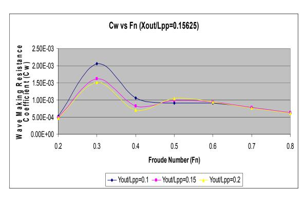
Figure 8. Wave Making Resistance Coefficient Results for  $X_{out}/L_{pp} = 0.15625$
