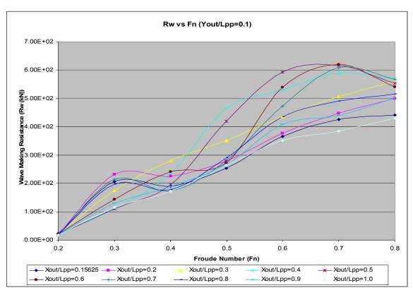
Figure 29. Wave Making Resistance Results for  $Y_{out}/L_{pp} = 0.1$
