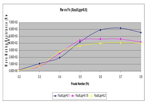
Figure 17. Wave Making Resistance Results for  $X_{out}/L_{pp} = 0.5$
