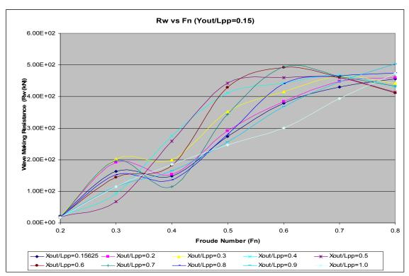
Figure 31. Wave Making Resistance Results for  $Y_{out} / L_{pp} = 0.15$
