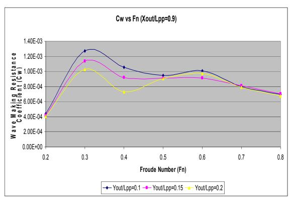
Figure 24. Wave Making Resistance Coefficient Results for  $X_{out}/L_{pp} = 0.9$
