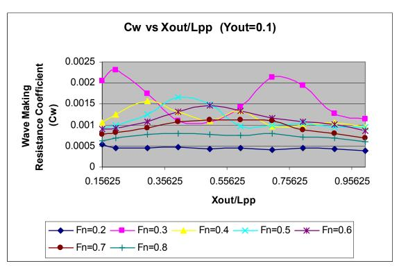
Figure 55. Wave Making Resistance Coefficient Results for  $Y_{out}/L_{pp} = 0.1$
