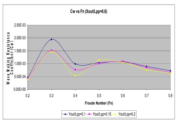
Figure 22. Wave Making Resistance Coefficient Results for  $X_{out}/L_{pp} = 0.8$
