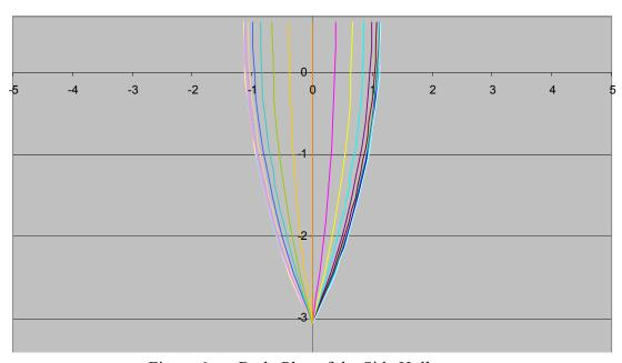
Figure 6. Body Plan of the Side Hull
