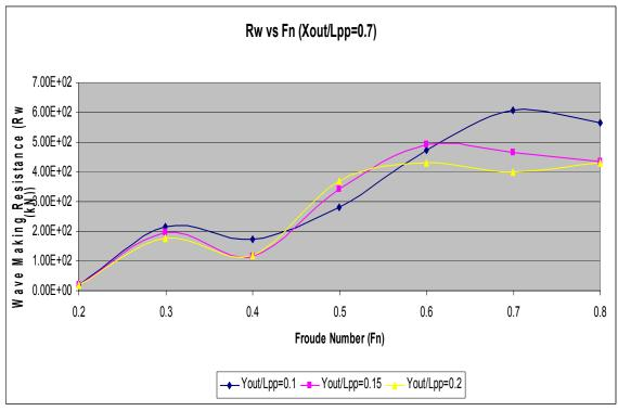
Figure 21. Wave Making Resistance Results for  $X_{out}/L_{pp} = 0.7$
