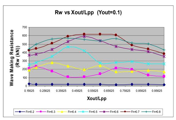
Figure 56. Wave Making Resistance Results for  $Y_{out}/L_{pp} = 0.1$
