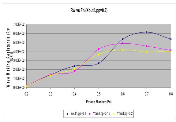
Figure 19. Wave Making Resistance Results for  $X_{out}/L_{pp} = 0.6$
