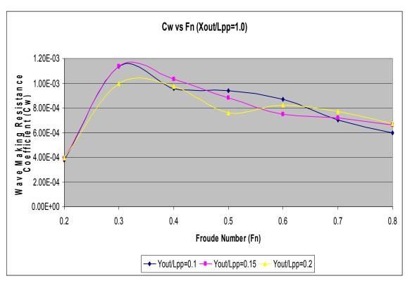
Figure 26. Wave Making Resistance Coefficient Results for  $X_{out}/L_{pp} = 1.0$
