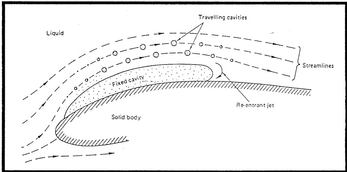
Figure 2.1 Fixed in travelling cavities
