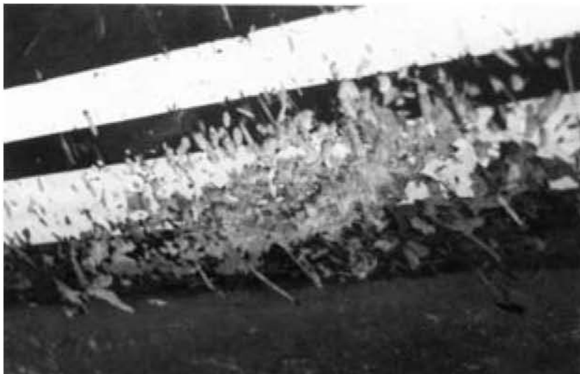
Figure 54 Abrasion damage to gelcoat and laminate
