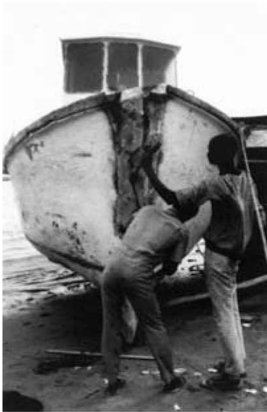
Figure 53 Collision damage to bow
