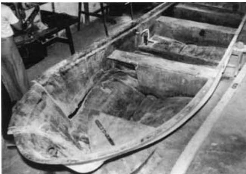
Figure 55 Severe impact damage to side
